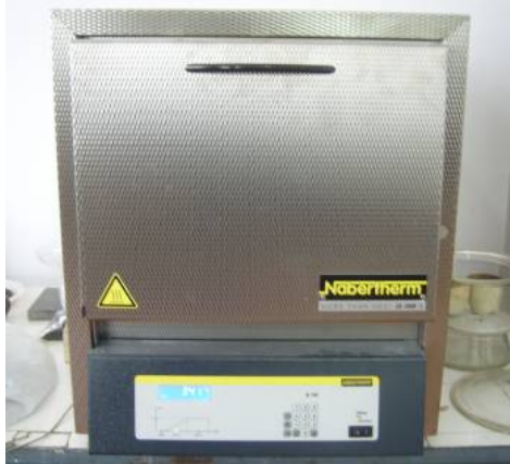
CUPTOR DE CALCINARE/ CUPTOR DE TOPIT NABERTHERM L15/12 B180A
